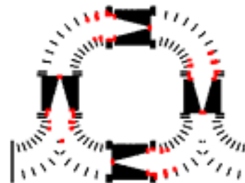
Figure 2. Snapshots of the trajectory of ions traveling two cycles around the cyclotron are plotted for three time points: 2.46, 3.39, and 18.60 ms. The left, center, and right columns correspond to ions with a 30% higher mobility than the compact [M + 3H]^{3+} ions of substance P, matched mobility ions (compact [M + 3H]^{3+} ions of substance P), and 30% lower mobility ions ( [M + 2H]^{2+} ions of substance P) at a drift field application period of 2.34 ms. Lenses of the cyclotron are shown in black, eliminated ions are in red, and transmitting ions are in blue.
